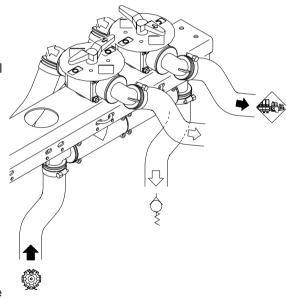
turned to "O" (closed). When spraying is to resume, select the Self-Cleaning Filter/operating unit. The other handles are turned to "O".
