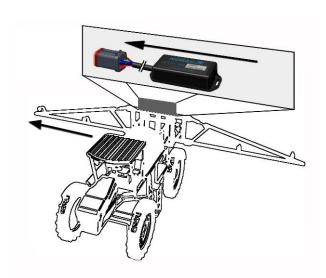
Figure 13: Roll Sensor Orientation - Connector Facing Right Wing
