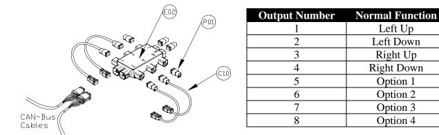
Figure 19: Valve Module
