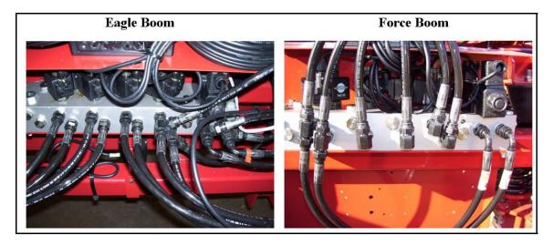
Figure 29: Location of Hoses on Hardi Valve Block
