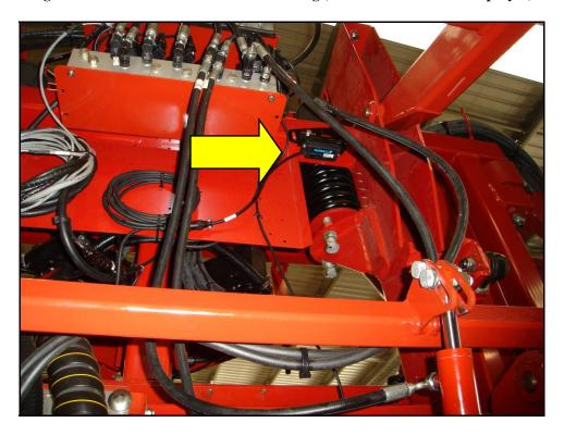
Figure 16: Chassis Roll Sensor Mounting (Viewed from the front of sprayer)
