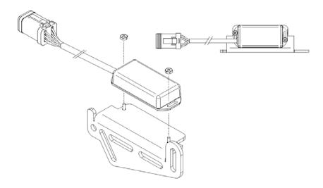
Figure 12: Mounting Roll Sensor to Bracket
