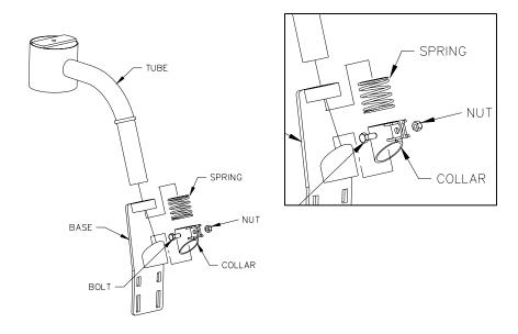
Figure 6: Breakaway Bracket Assembly
