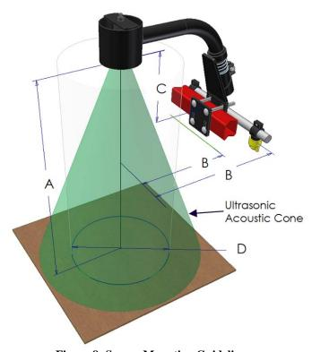
**Figure 8: Sensor Mounting Guidelines**
