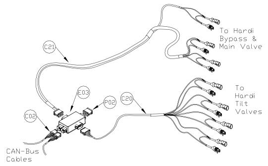
**Figure 23: Input Module Connections**
