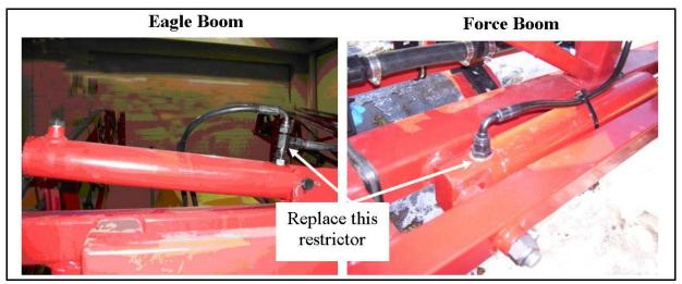
Figure 28: Restrictor to be replaced on the tilt cylinders
