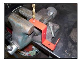
Figure 10: Drilling the main lift sensor bracket
