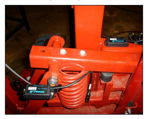
Figure 17: Roll Sensor Mounting (Viewed from the rear of sprayer)
