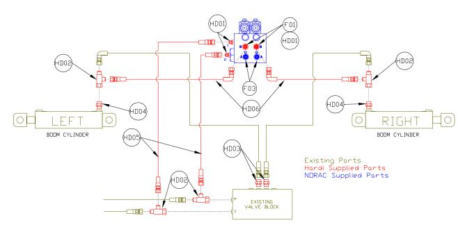
Figure 3: HD03 Hydraulic Plumbing: Single Acting (Force Boom)
