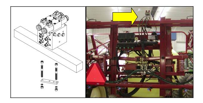
Figure 27: Valve Block Mounting
