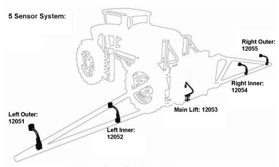
Figure 7: Sensor Serial Number Arrangement
