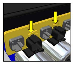
Figure 21: Valve Module Bracket Installation
