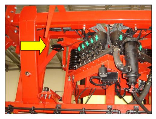
Figure 15: Boom Frame Roll Sensor Mounting (Viewed from the rear of sprayer)
