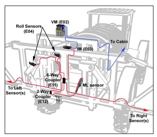
Figure 24: UC5 Module Locations and Cable Connections
