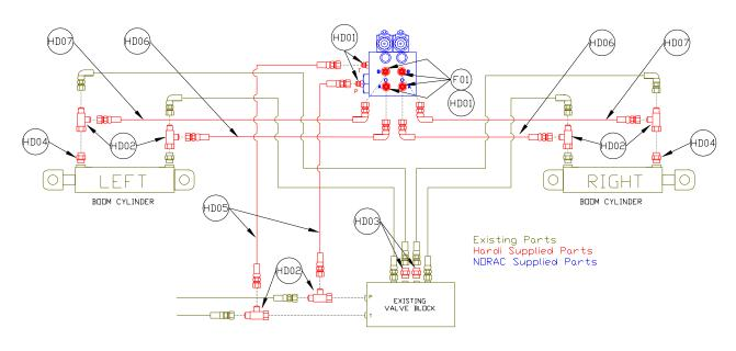
Figure 4: HD03 Hydraulic Plumbing: Double Acting (Eagle Boom)
