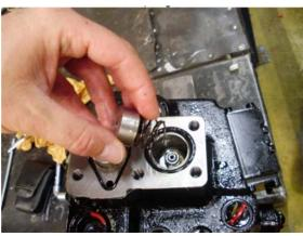
• Remove the valve with needle nose pliers.
