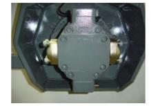
• Remove the 4 screws on the flange.
