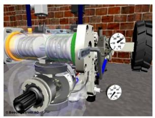
• After balancing pressure switch to 580psi (40 bar) manometers for finer adjustment.
