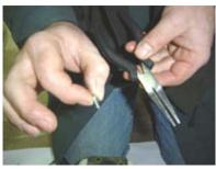
• Tighten the screw in the plug and remove it with the pliers.
