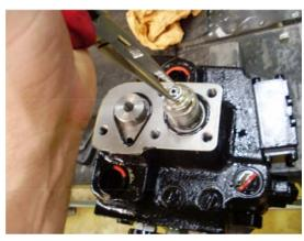
• Remove the nut at the end of the valve.
