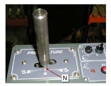
2. Maintain the potentiometer lever in position using a 3mm drill bit as shown.
