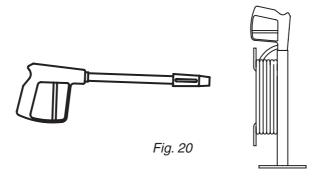
A spraygun with adjustable spray pattern and 25 or 50 ft. of hose for spraying fence row or spot spraying a small area can be installed onto your sprayer. A handy hose wrap and spraygun holder can be conveniently located on the sprayer to transport the spraygun.
