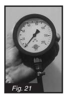
A large and easy to read 4" pressure gauge is available to replace the standard 2-1/2" gauge.
