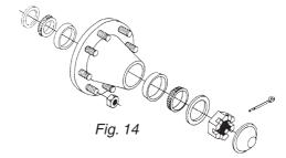
After 1000 hours or once a year, the axle bearings should be repacked with new grease.
