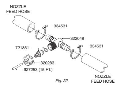
A remote nozzle pressure gauge may be added by ordering the parts listed above. To install, cut one of the nozzle feed hoses at the rear of the sprayer and insert the tee (#322048) as shown above. The hose (#927253) is then run to the pressure gauge (#284277) mounted on the magnetic base (#10536803). The magnetic base may be placed near the operator to better monitor the pressure at the nozzles for more accurate control of the application rate.
