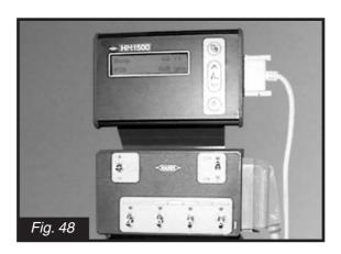
The HARDI® Monitor 1500 monitors the application rate. When used with the electric control unit switch box, correct area covered and up to 8 spray boom section control is possible. Components can be added for your individual requirements to control your operating unit, and optional equipment.
