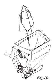
11. If the chemical container is empty, it can be rinsed by using the Bag & Bottle Rinse (optional). Fit the bag bracket and place the powder bag over the multi-hole nozzle and press the lever (B) (Fig. 20).
