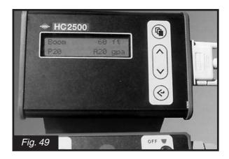
The HARDI® Controller 2500 permits automatic control of the application rate. This allows you to concentrate on driving as the rate is automatically maintained by the HC 2500. Press the "up" or "down" arrow key to change the application rate. Easy, quick and simple. Up to 8 spray boom section control is possible.
