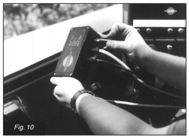
12-volt junction box for 12-volt hook-up: EC or EVC controls, HARDI® HM1500/HC2500, Foam Marker, Boom Hydraulic Controls, etc.
