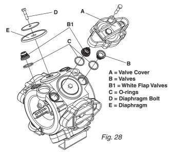
Diaphragm pump overhaul kits (valves, seals, diaphragms, etc.):
