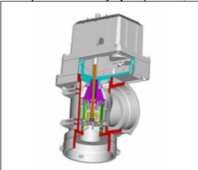
Figure 3 Pressure regulation valve
