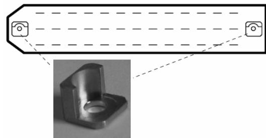
The dowel is set as when viewed into the plug on the cable. Re-coding the dowel allows switching from liquid to hydraulic and vice-versa.
