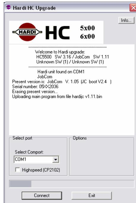
When the upload of the new software has started, diode N28 and D27 will start to flash together with the watchdog.
