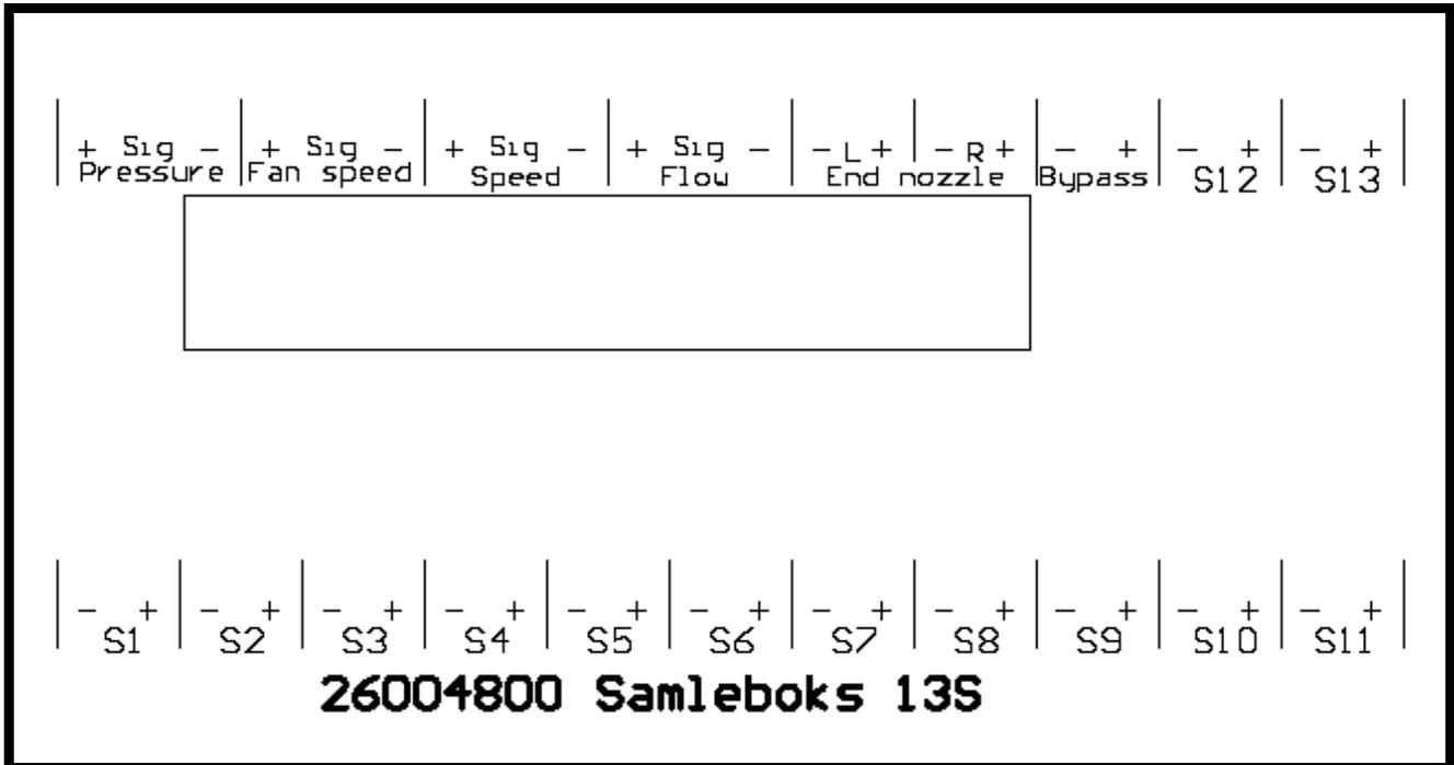
Picture 17 PCB for section valves "New Commander" (13 sections PCB)
