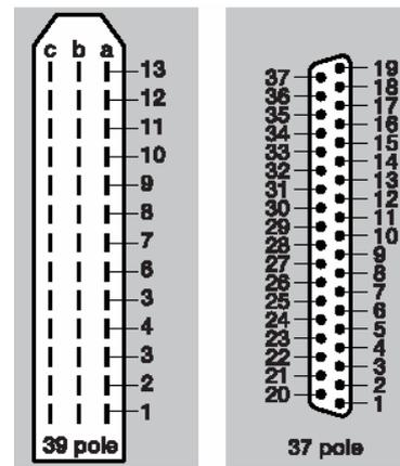
The 37 - 39 pole connector has the same wiring combination for the hydraulic and fluid system. Therefore the cables are coded with a dowel so they can not be connected to the wrong box.
