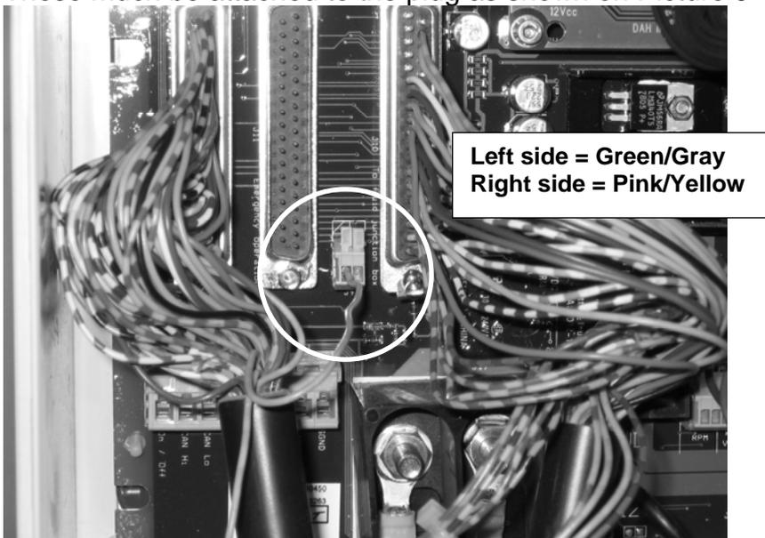
**Picture 9 Connection of the two wires from Spray box cable**
