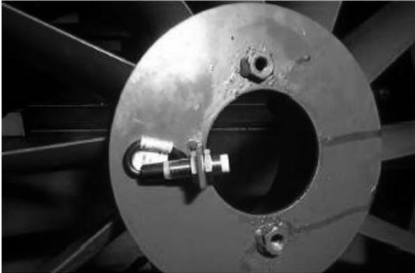
**Picture 7 Fan speed sensor**
