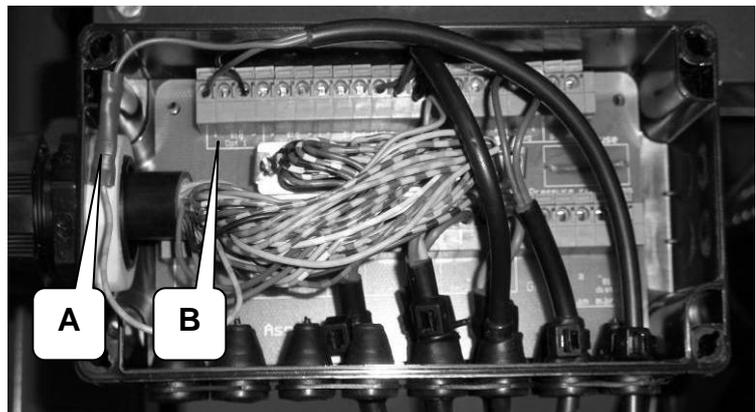
The cable from the Spray box has two loose wires which are not connected in the Jobcom. These must be attached to the plug as shown on Picture 9
