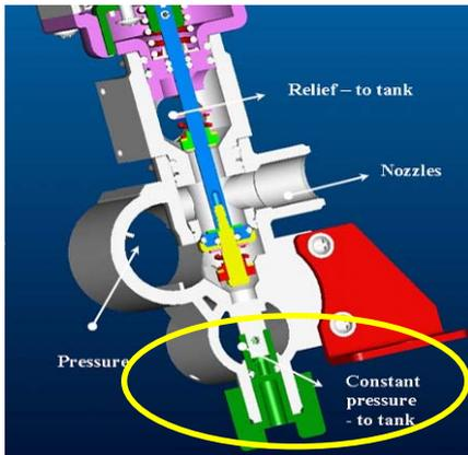
Picture 11 EVC with the equalization system
