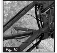
**Note:** The boom also has a rear transport lock which automatically engages and disengages during folding and unfolding.
