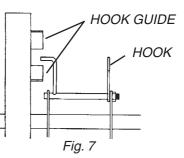
acting outlet until the control arm of the hook appears between the two flat bars of the hook guide (Fig. 7). Be careful not to bring the control arm past the opening on the hook guide.
