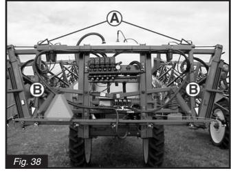
Center section cables work together to keep the center frame square to the Paralift<sup>TM</sup>, whether folding the boom in for transport or when spraying with one side raised and folded (HZ Only).
