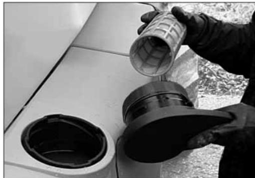
To drain the filter housing:
