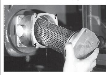
NOTE: When cover and filter are removed quickly, a built-in valve will prevent oil tank from being drained. Appx. 1½ I of oil will be wasted during filter change - retain waste in appropriate container.
