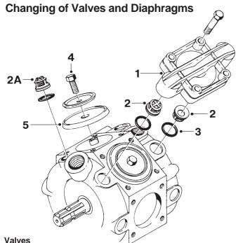
Remove valve compartment 1. Before changing the valves 2 note the orientation of the valves so that they are replaced correctly.
