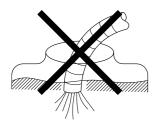
WARNING! DO NOT LET FILLING HOSE ETC. ENTER THE TANK. KEEP IT OUTSIDE THE TANK, POINTING TOWARDS THE FILLING HOLE.
