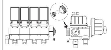
Remove the 2 bolts holding the on/off-pressure valve unit to the bracket **A**, unscrew the union nut **B** and pull the on/off-pressure valve away from the distribution valves.
