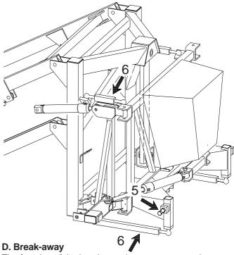
The function of the breakaway is to prevent or reduce boom damage should it strike an object or the ground. The break-away can not be adjusted, but shall only be kept greased (see section "Lubrication").
