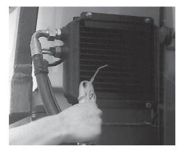
2. Oil cooler Clean oil cooler using
