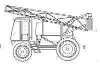
axles with hydraulically activated brakes in oil bath. The cabin is of a fully closed type with ventilation air, filtrated through carbon filters for driver's safety. The cab can be equiped with air-conditioning and heater/defroster is factory fitted optional extra. OLH 20, 21, 24 or 28 m fully hydraulic operated and pendulum suspended boom is standard.
