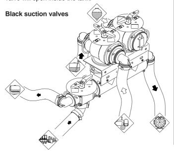
Turn the handle so the arrow points towards the selected optional equipment. The handle is turned back when you want to aspirate from the main tank. If 2 valves are fitted, eg. Filling device and Rinsing Tank, select optional extra and turn the other valve to "O" (closed). To resume aspiration from the main tank, the arrow must point towards the main tank. Remaining valve must be closed.
