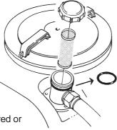
Nozzle blockages do not occur whilst spraying. Long life of pump. A blocked suction filter will resume in pump cavitation.
