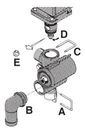
Then unscrew the screw  ${\bf D}$  and replace the valve cone  ${\bf E}$ . Reassemble in opposite sequence.
