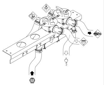
To select the optional equipment, the handle is turned so the arrow and thereby liquid is directed to the optional extra instead of to the self-cleaning filter/operating unit. When spraying is to resume, turn the handle so the selfcleaning filter/operating unit is selected.
