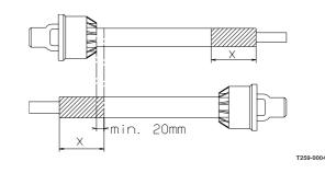
**NOTE!** The shaft must always have a minimum overlap. The size of this overlap depends on the pump model:
