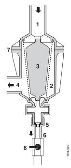
Ball check valve (8) should normally be open, but can be closed in situations where return flow is to be avoided.
