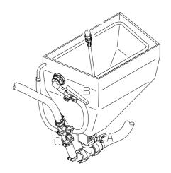
**NOTE!** The scale in the hopper can only be used if the sprayer is parked at level ground! It is recommended to use a measuring jug for best accuracy.
