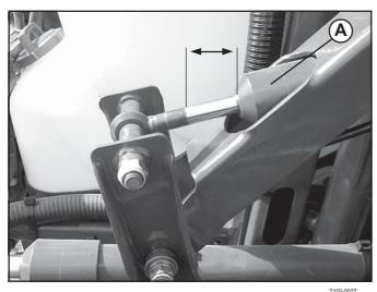
Boom wing should be horizontal. If not, align boom wing by means of axle (**B**). See below.
