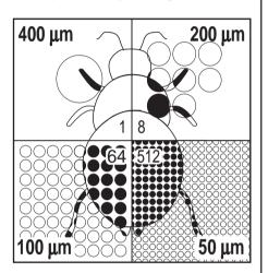
Halving one 400 mm drop produces 8 drops of 200  $\mu$ m. With these smaller drops, it is possible to cover about twice the area.
