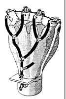
The majority of nozzles for mistblowers are made of ceramic material. This ensures long life even at high working pressures but even so they do wear. If nozzle output is more than 10 % in relation to the theoretical (table) value, the nozzle should be replaced.
