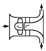
Centrifugal fans produce high air speeds and high air pressures but low air volumes. The blower typically has hoses and spouts to localize the air.
