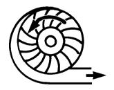
The blower housing may direct the air out to both sides or to one side.
