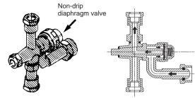
Flip-over double nozzle holder with non-drip diaphragm valves
