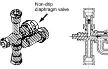
Flip-over double nozzle holder with non-drip diaphragm valves
