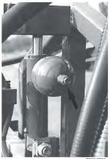
When the damper nitrogen pressure is correct the distance L must be 40-50 mm. To adjust the distance:
